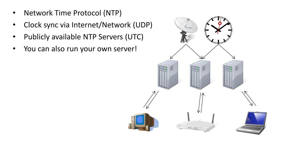
Packet delay is estimated to reduce clock skew
